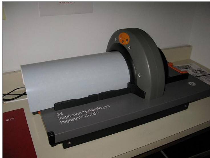
Figure 18. Portable Computed Radiography Scanner Model CR 50P (34)
