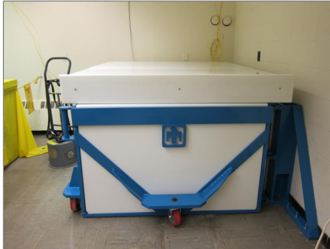
Figure 6. Polyethylene Chamber for Shielding and Storing the Neutron Source
